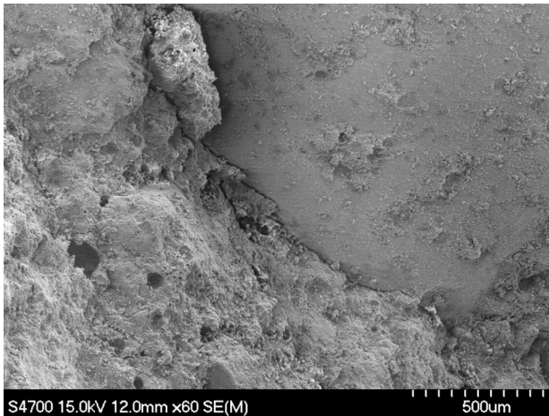
Figure 12. Interface between aggregate and geopolymer (concrete, fly ash:aggregate = 1:4.7, w = 0.37 , fractured flat, 28 days).
