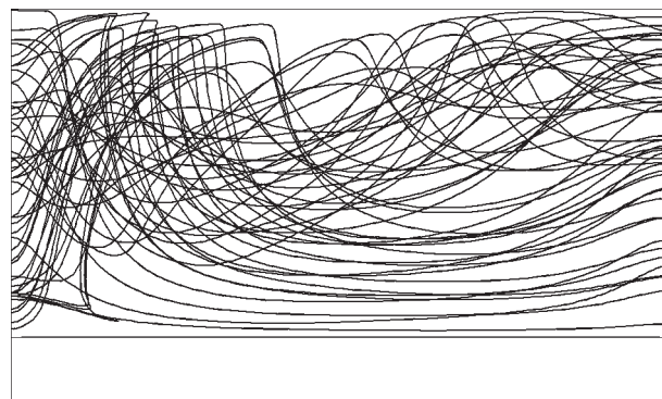
Figure 4. The projections of the representative 25 melt trajectories into the longitudinal vertical (axial) plane in the TV glass melt with the helical melt flow. The average temperature was kept at a temperature of 1450°C, the value of the transversal temperature and gradient was 25°C/m and the ratio of the transversal to the positive longitudinal temperature gradient was 5 ( u_D = 0.654 , u_F = 0.705 ).
